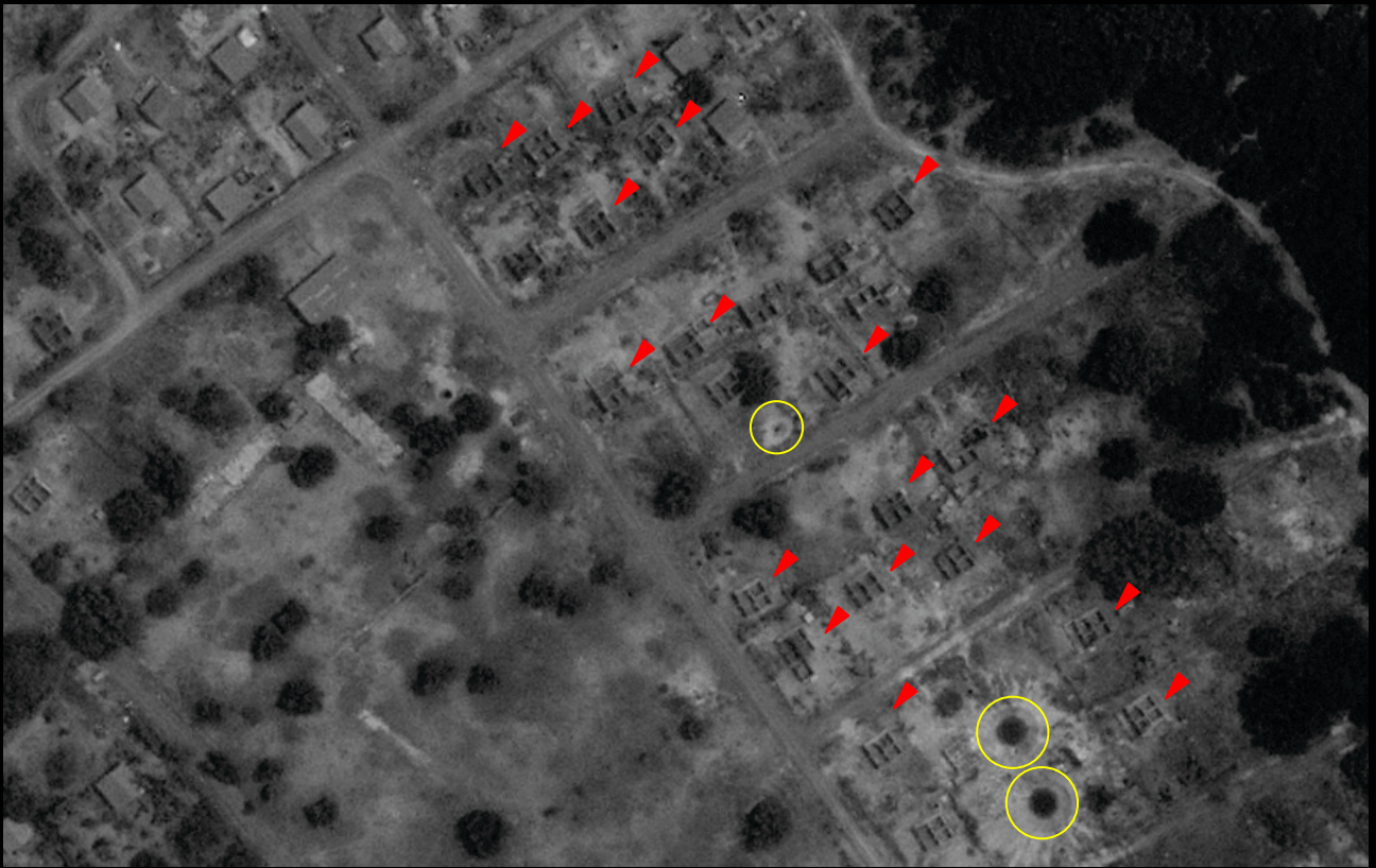
Figure 9.4-24: Damage to buildings due to artillery. Destroyed buildings generally have load-bearing interior and exterior walls left intact with the roof removed. Area Vadduvakallu – Source: earth.google.com
